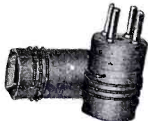
MIDGET ULTRA SHORT-WAVE R-39 FORMS and COILS
