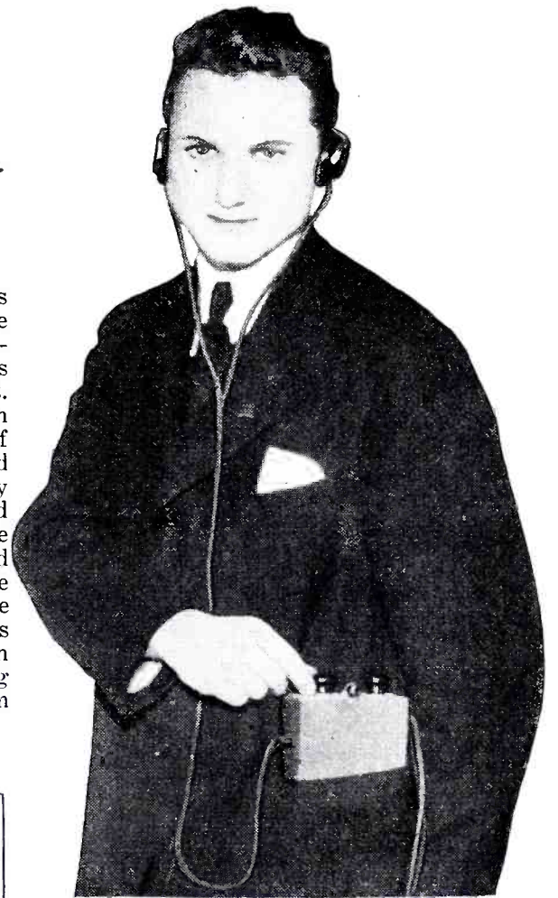
Max D. Pearlman tuning in a station on the "pocket receiver." The choice of short or broadcast waves is provided, and with a good pair of phones some very excellent results have been obtained.
